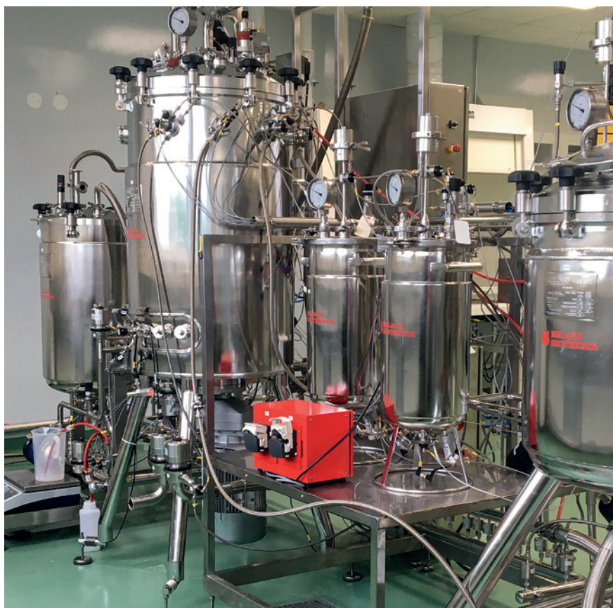
Production-scale fermenter from Belach Biotechnik
